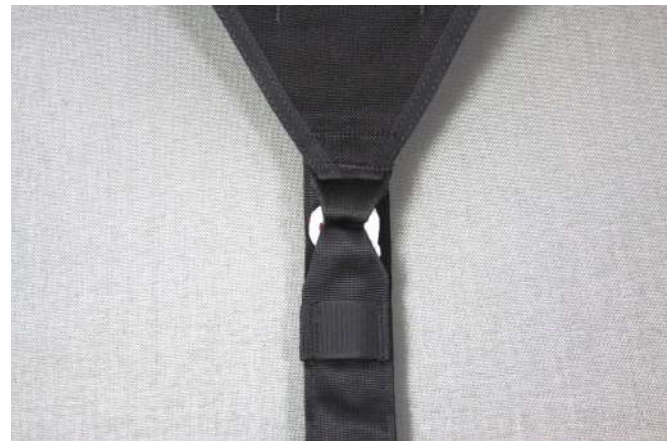
The drogue bridle and the deployment bag replaced.
