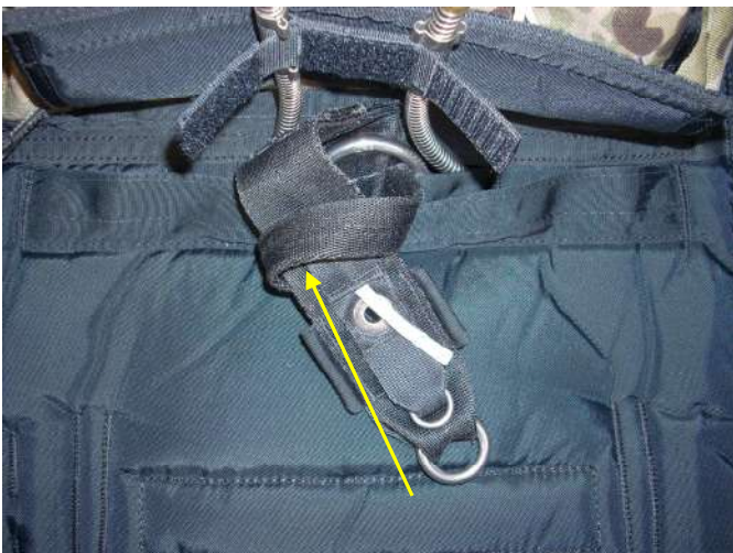
Pass the 3-ring drogue riser back through the lark's head knot.
