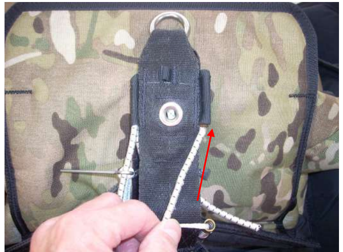
Insert the elastic into the front channel of the drogue 3-ring riser.
