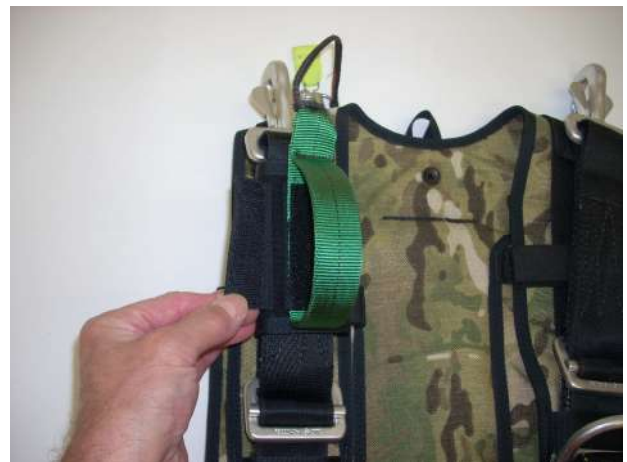
Close the Velcro covering of the handle pocket over the examiner's handle.
