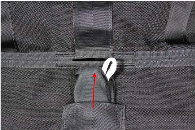
Insert the drogue bridle into the slot on the bottom of the deployment bag.
