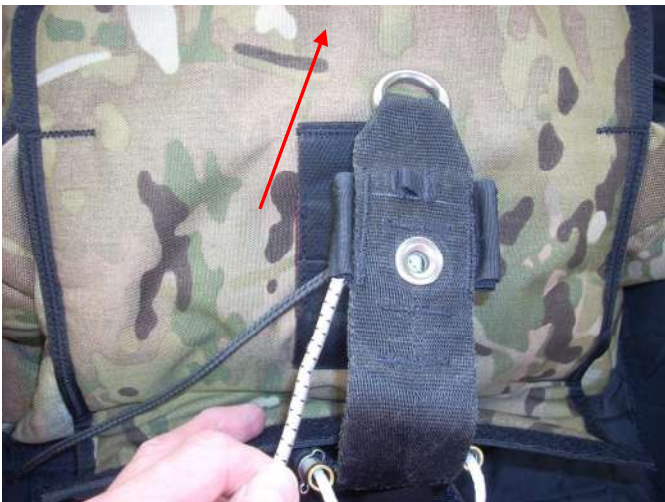
Insert the elastic into the back channel on the 3-ring drogue riser.
