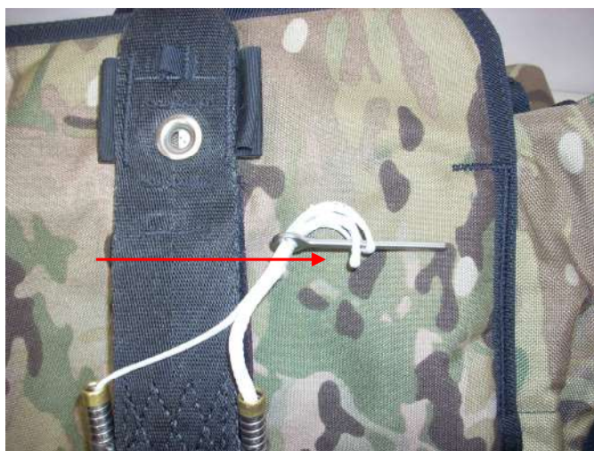
Pass the straight pin through the loops of the release lanyards.
