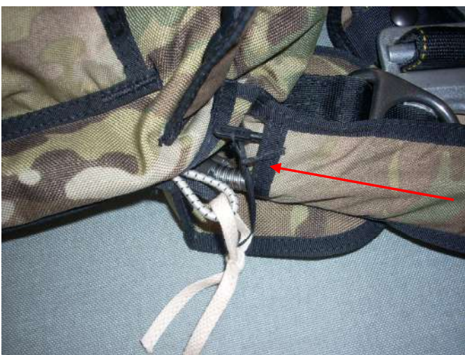
Insert a .22 rifle cleaning rod into the opening on the right side of the handle sleeve. Attach the retractable connector loop to the cleaning rod.
