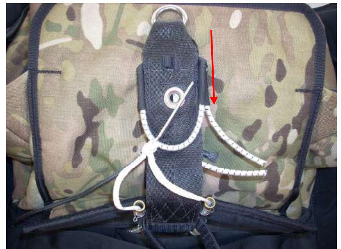
Loop the elastic up and into the back channel.
