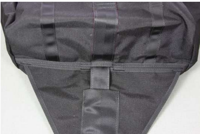
Insert the drogue bridle into the slot on the bottom of the deployment bag.
