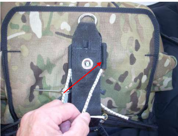
Completely remove the elastic from the channels on the sides of the riser.
