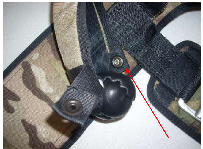
Unsnap the right side drogue release handle from the right leg strap.
