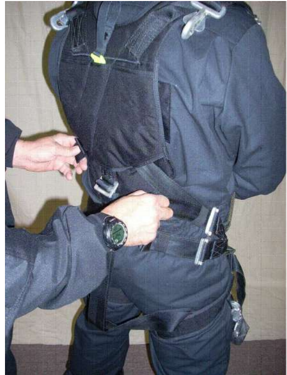
Take the slack out of the back strap. Make sure that it sits above the buttocks.
