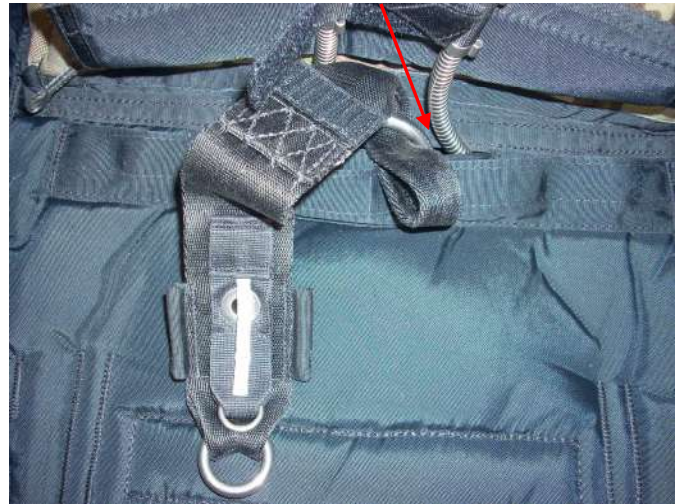
With the Type IIA loop and mini ring facing up, pass the loop end of the 3-ring riser through the large ring of the internal harness.
