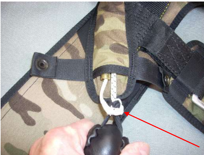
Pull the right side release hacky to find the right release lanyard attachment knot.
