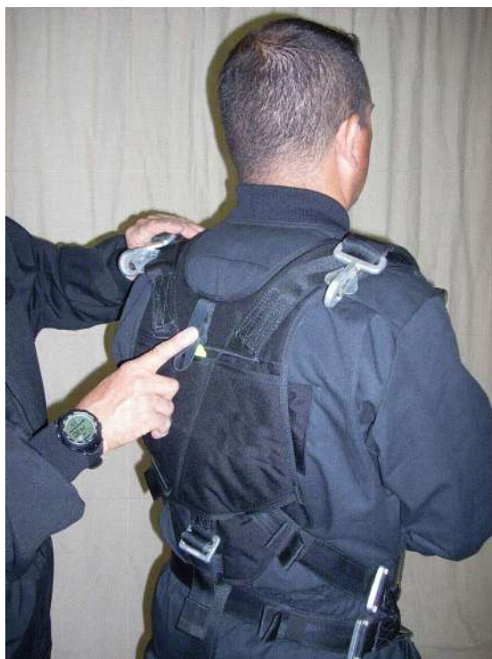
Confirm that the harness yoke sets just below the back of the neck.
