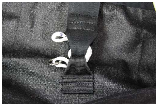
Open the soft link completely.
