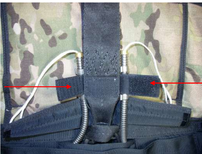
Mate the hook Velcro on the 3-ring drogue riser to the pile Velcro on the release housings.
