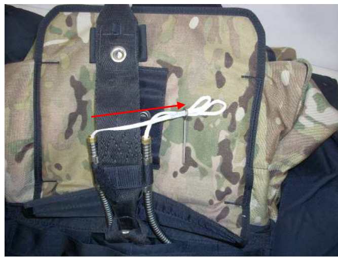
Pass the Two (2) release lanyards through the eye of the straight pin.
