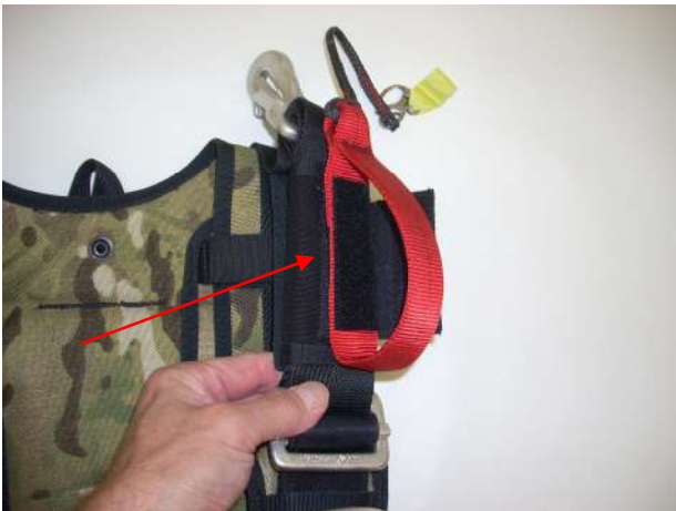
Mate the Velcro of the examiner's handle to the Velcro of the handle pocket.
