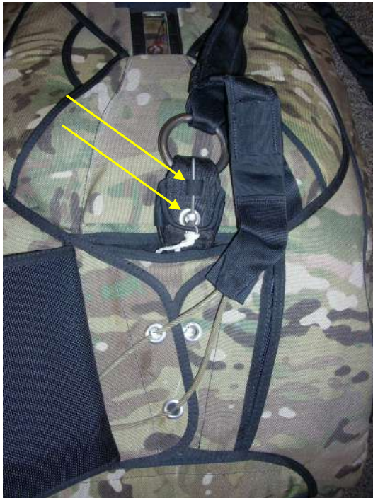
Secure the loop with the straight pin and tuck the pin end under the tape as shown.
