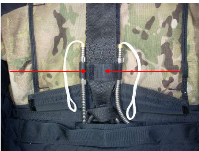
Mate the pile Velcro tab to the hook Velcro of the 3-ring riser, then the hook Velcro tab to the pile Velcro tab.
