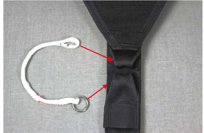
Pass a soft link through the loops of the drogue bridle and the deployment bag.
