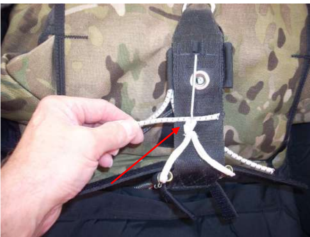
Remove the elastic from the straight pin.
