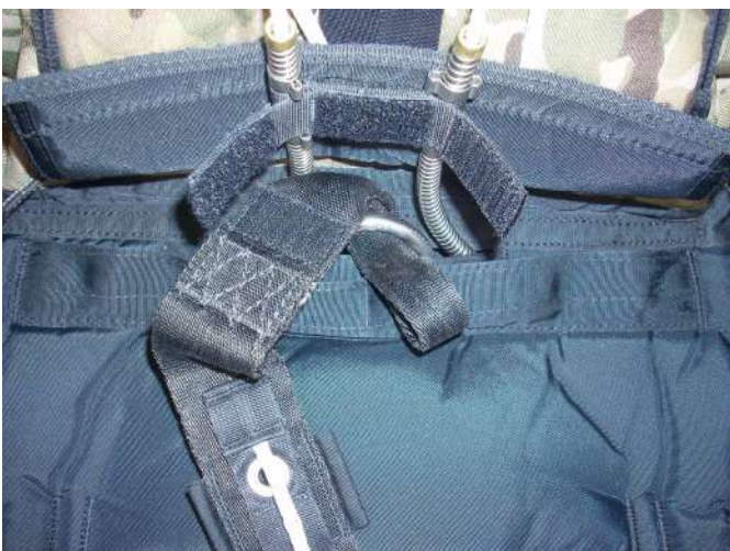
Pass the 3-ring drogue riser back through the lark's head knot.
