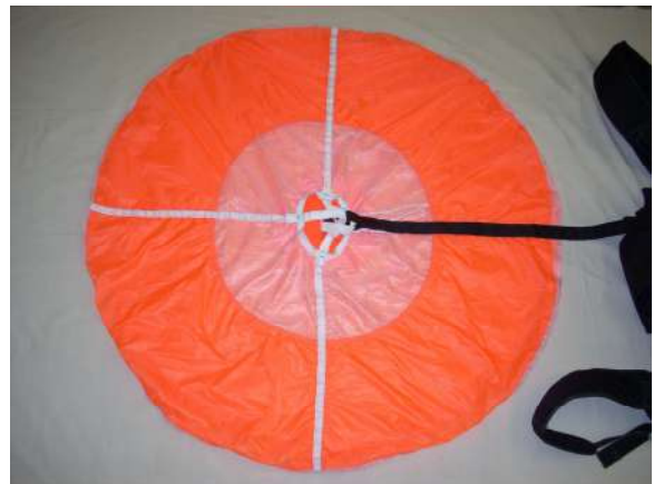
With no twist in the bridle, lay the drogue out flat on its top, mesh side up, handle down.
